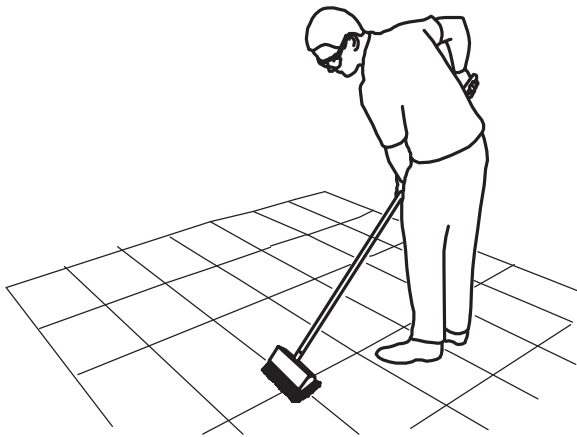
Scrub floor and grout lines with brush.
