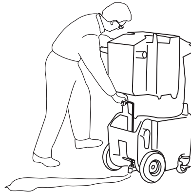
Open spigot and apply solution to floor.
