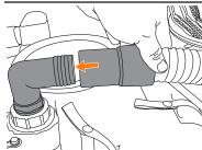
Ensure elbow hose is connected at top of machine.
