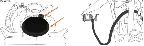
Note the location of the Sight Gauge on the side of the Water Tank. Use the Sight Gauge feature to see how much water is in the machine. If water is low, ensure you refill the tank by using the fill port. The Sight Gage will help see the water level, do not overfill or overflow from the tank will occur.
