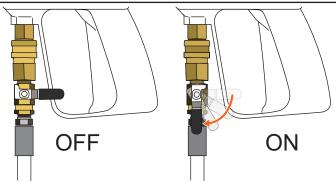
To turn Spray Lance off or on, switch the valve connected to Spray Lance as shown. The Spray Lance is connected to the Spray Line.
