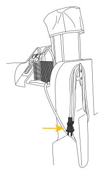
Lower Power Pack onto bracket slide, lowering it down into place.
